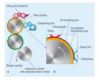
Fig. 1. Components of a printing unit.
